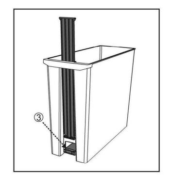
3 Bring the end of the push-rod down to meet the 'cup' at the end of the pedal as indicated above.
