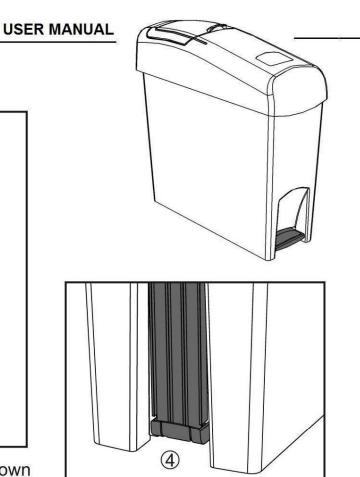
Press down on the push-rod so that it 'snaps' into the pedal and locks in place as shown above.
