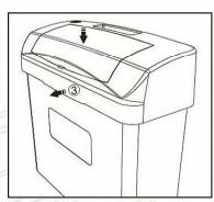
③ Pull out the front face of the cover and push the cover down, then release the front face.
