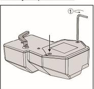
① Unscrew the 2 Allen bolts with a 3mm Allen key.
